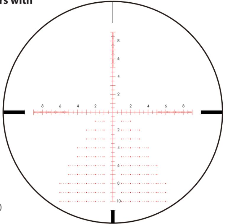
Either the vertical or horizontal scale can be used to range for your target. Try to read mils as accurately as possible. Reading MILs in 1/10 accuracy or MOA in .25 MOA accuracy will provide a more accurate range to the target. Therefore, using the end of either the horizontal or vertical scale will provide more accurate measurements.
