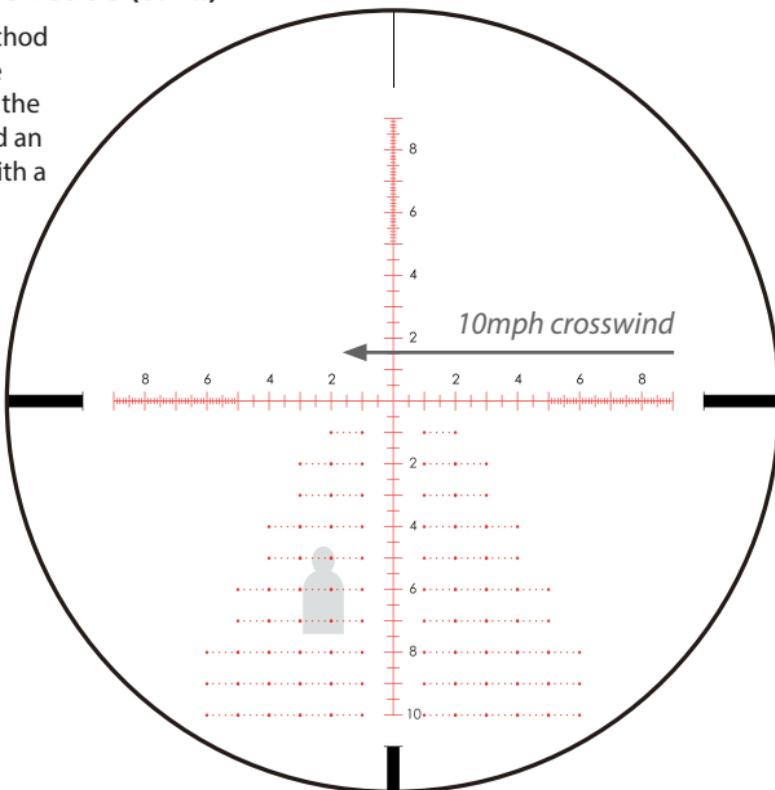
Determining a target lead requires knowing target speed, target distance, wind speed, and bullet flight time to target's distance. Also, correcting weapon cant is a critical step to ensure accuracy for target leads. Again, it is recommended to utilize a ballistic calculator to increase your shooting effectiveness. Finally, mastering this level of marksmanship takes experience. It is also recommended to further your knowledge and study ballistics manuals and shooting guides.
