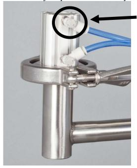
• Filling volume is changing depending from volume in the container Solution: rotating cylinder must be fully extended (air supply to the filling machine) and check that opening in the rotating valve is inline. Loosen two bolts and adjust lever.
