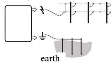
Fence systems may be operated independent of each other at the fence connections (5 or 6).
