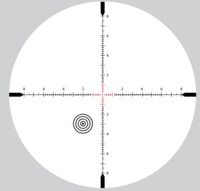
1.95 mil lead holdover for a moving target traveling at 2 mph from left to right at 500 yards. Bullet flight time is 1 second during which the target traveled 2.94 feet. No wind.
