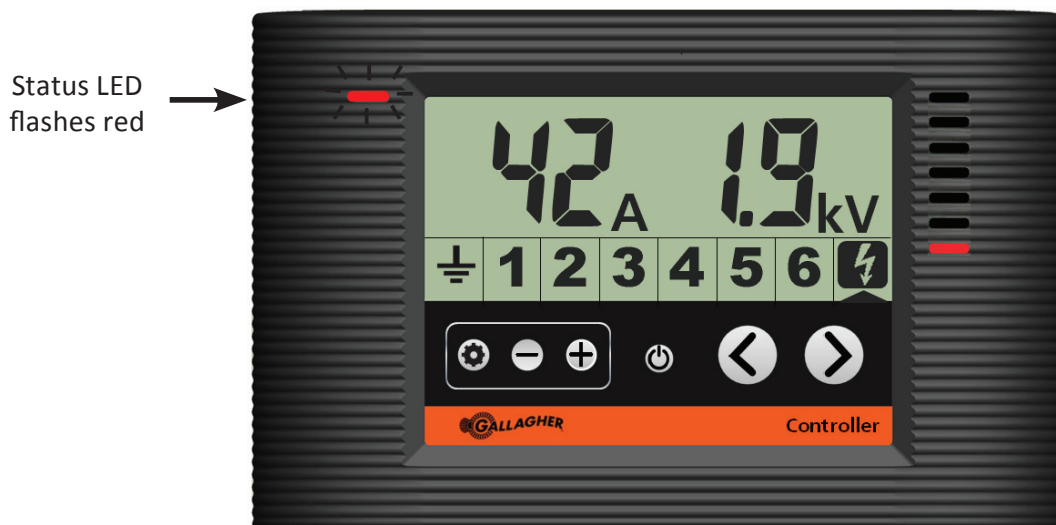
Controller showing the energizer in output alarm
