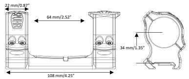
The SCT-6006 Hunting Mount features one Spuhr Interface™ Top Cover, which can be installed as to position any of more than 40 different accessories in either the 12 or 3 o'clock position.
