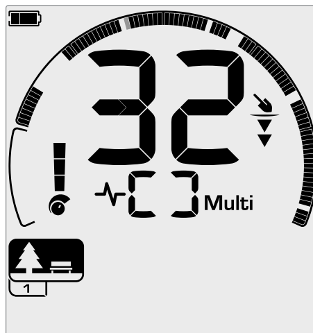
Example showing the detection of an accepted non-ferrous target with a Target ID of 32. Segment 32 on the Discrimination Scale will flash.
